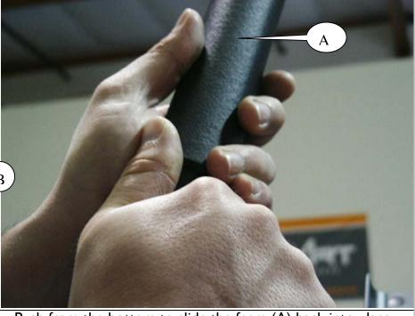
Push from the bottom to slide the foam (A) back into place. Do not spray hairspray into the space between the foam and metal, as it promotes rusting. Blowing compressed air from the bottom can help in getting the foam in place.
