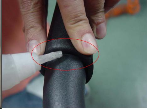
Roll up a small part of the foam, and squirt a dab of quick-dry glue (Cyanoacrylate Adhesive), then put the foam back in place.
